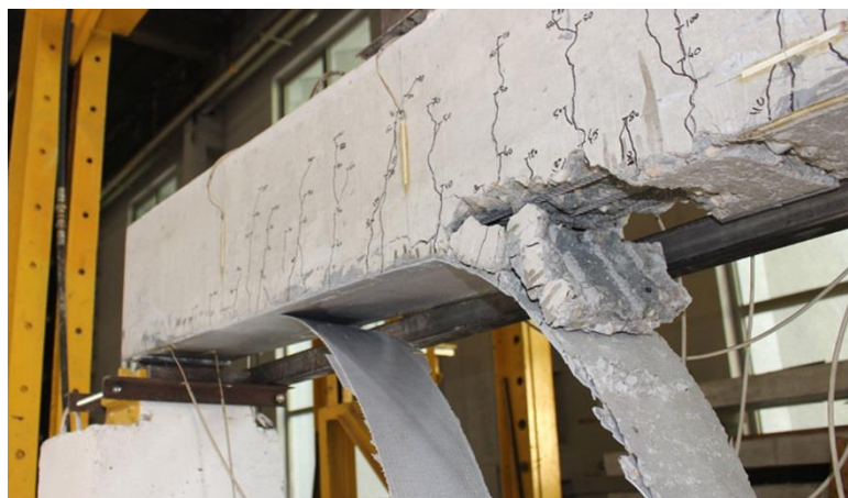
Figure 5. Debonding failure of beam strengthened with two layers of SRP textile composite.
