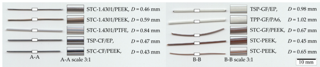
Figure 6. Selection of investigated specimens. Abbreviation: carbon fibre (CF), epoxy resin (EP), glass fibre (GF), shrink tube consolidation (STC), thermoplastic pultrusion (TPP), thermoset pultrusion (TSP), polyamide (PA), polyether ether ketone (PEEK), polytetrafluoroethylene (PTFE). The detail views A-A and B-B of the different specimens were visualised with a triple magnification.
