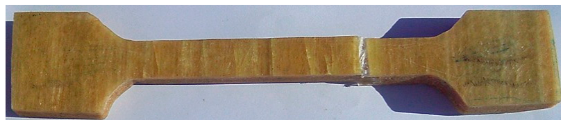
Figure 9. Tensile specimen fracture mode.
