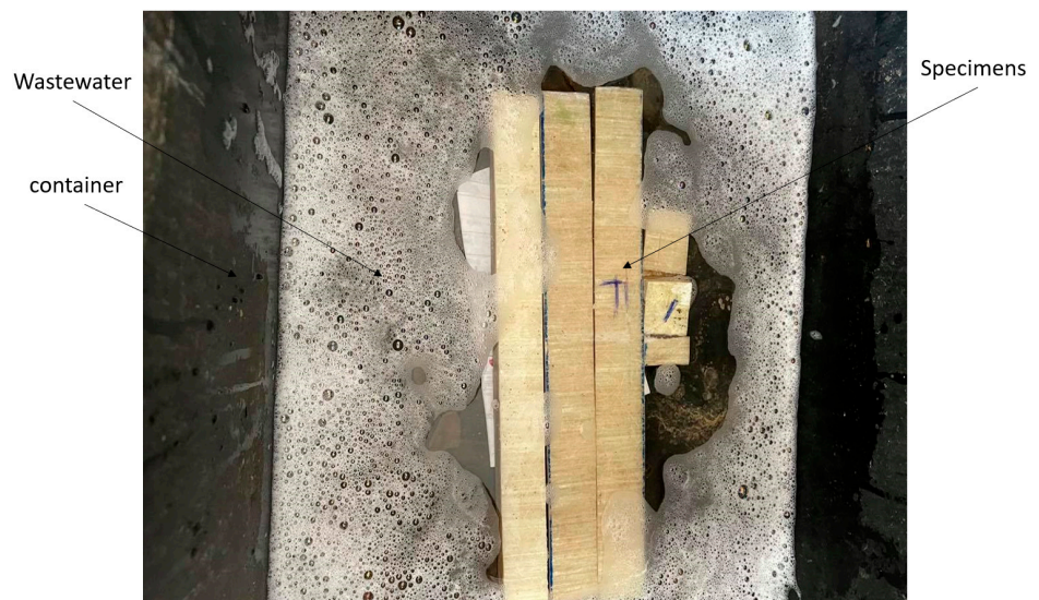
Figure 2. Chemical treatment to preconditioning the GRP pipes material.
