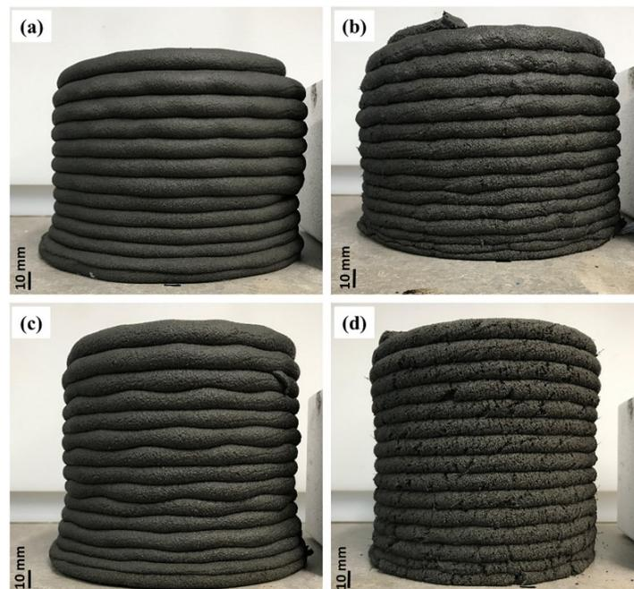
**Figure 16.** Buildability of geopolymeric printable composites reinforced with nano-clay additives and PVA fibers (reproduced with permission from Chougan, M. et al., *Materials and Design*; Elsevier, 2021).
