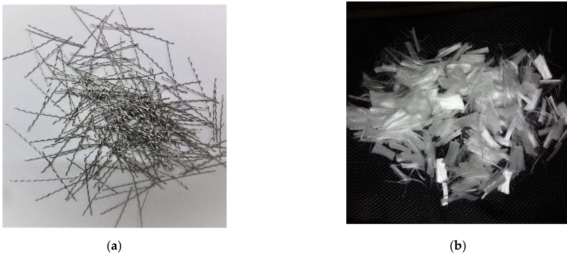
Figure 1. Fibres used: (a) Crimped steel fibres; (b) Polypropylene fibres.
