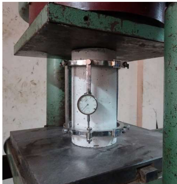
Figure 3. Modulus of elasticity test setup.
