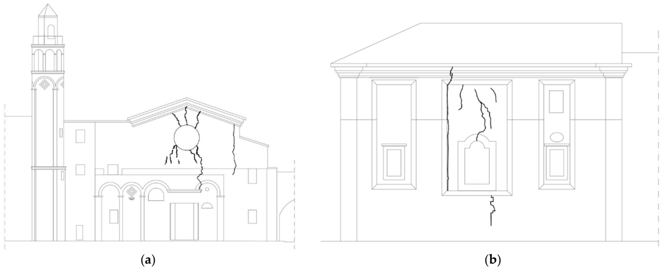
Figure 16. Graphic representation of the crack pattern on the façades: (a) main façade; (b) rear façade.
