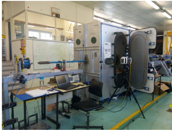
Figure 2. Picture of the setup for the gas gun and chamber.
