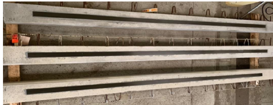
Figure 1. Samples of composite/RC-beam adhesively bonded assemblies.
