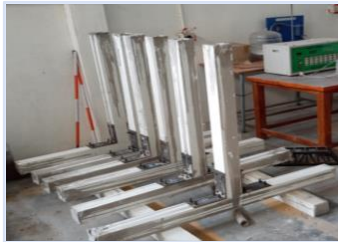
Figure 5. The casting of GFRP beam-column specimens.
