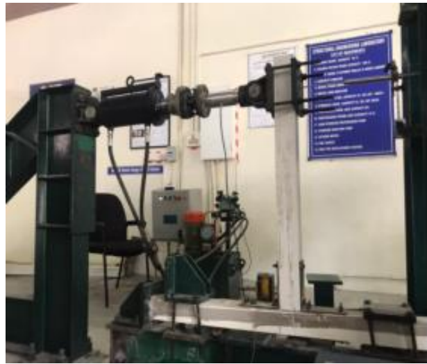
Figure 7. Experimental setup for lateral loading on beam-columns.
