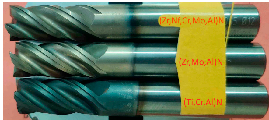
Figure 1. General view of the coated milling cutters (after milling).
