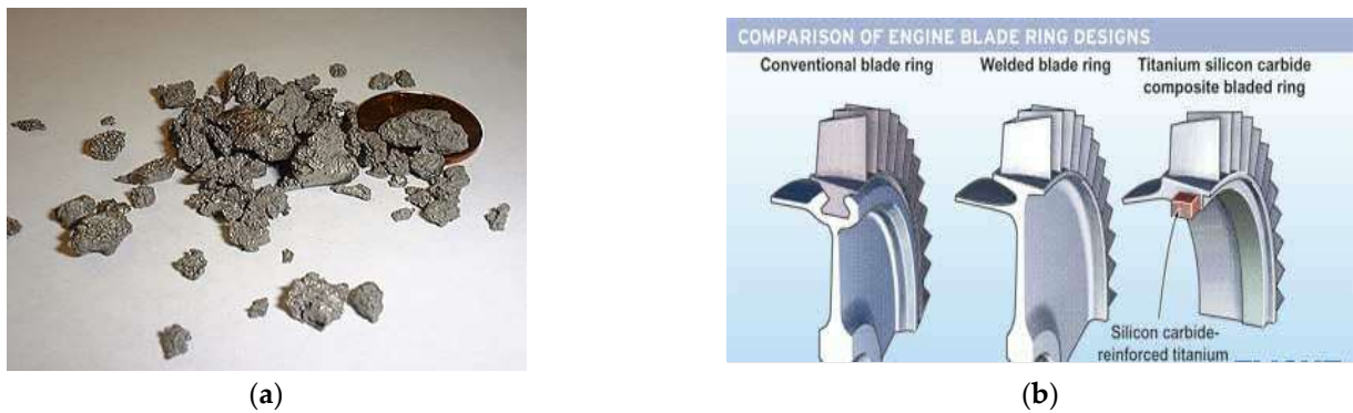
Figure 2. (a) Titanium Sponge (b) TMC Engine blade ring of aircraft [29].
