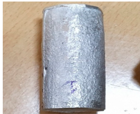
Figure 1. Fabricated hybrid composite sample using stir casting process.
