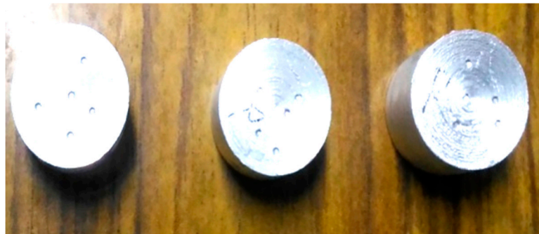
Figure 2. Hybrid composite specimens after hardness test.
