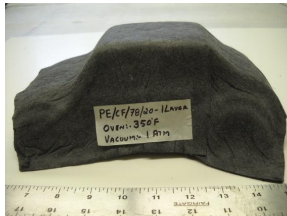
Figure 11. Forming via SDF exhibited optimal draw and consolidation.
