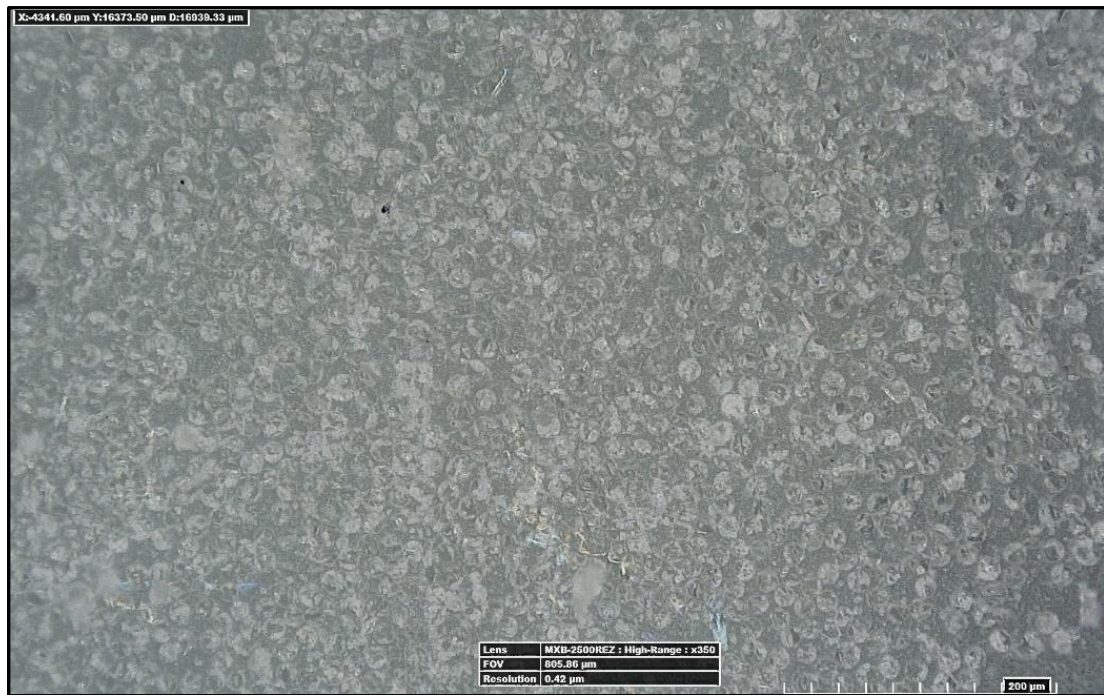
Figure 7. R-glass FRP plate with a (bottom; \times 350 magnification) transverse and (top; \times 350 magnification) hoop fiber orientation after a week of exposure to pH 10.0 aqueous solution.
