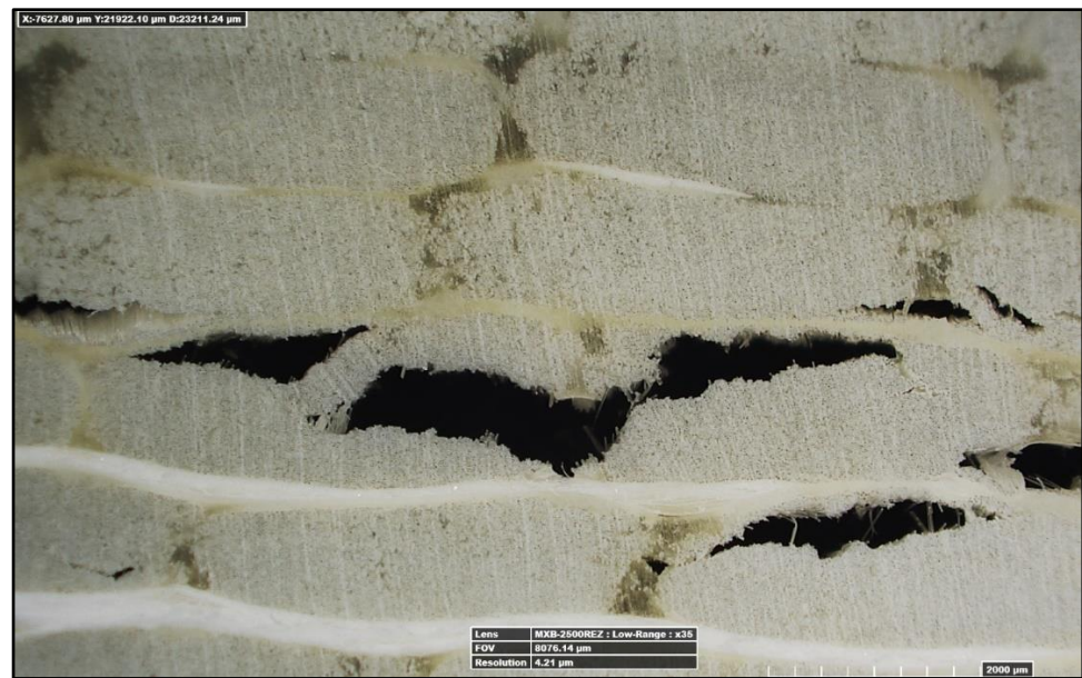
Figure 4. R-glass FRP plate with a (bottom; \times 35 magnification) transverse and (top; \times 140 magnification) hoop fiber orientation after a week of exposure to pH 1.7 aqueous solution.
