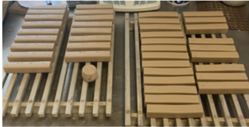
Figure 5. Dried samples before being placed to the electric laboratory kiln.
