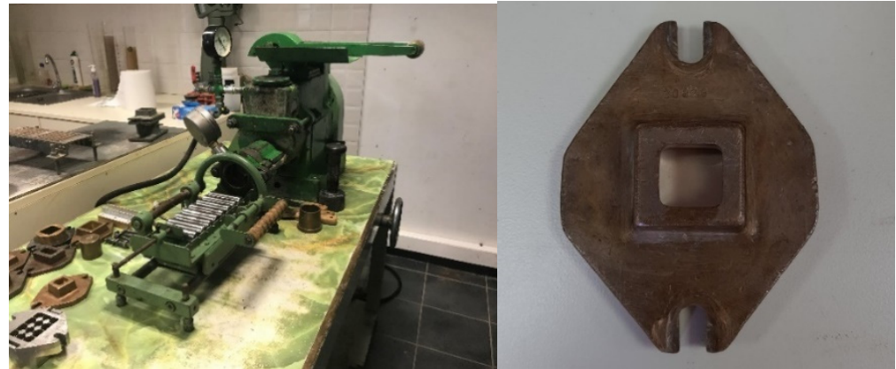
Figure 4. The extruder and the sample mouth of the extruder.
