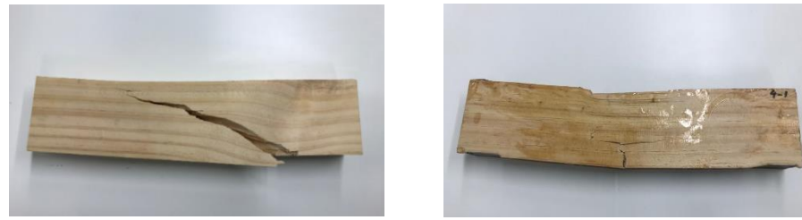
Figure 5. A 40 \times 80 sample piece from benchmark case 1 (left) compared to the most promising reinforced 40 \times 80 sample Case 4 (right) after loading.
