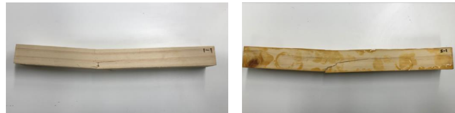
Figure 6. A 40 \times 40 sample piece from benchmark case 1 (left) compared to the most promising reinforced 40 \times 40 sample Case 5 (right) after loading.
