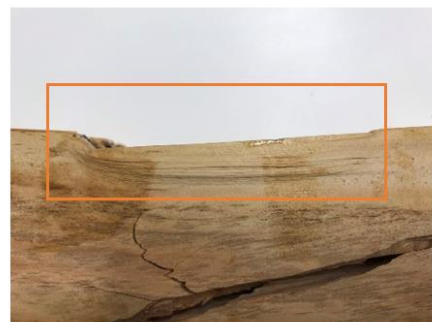
Figure 4. A slow deformation is seen at the compression (top) zone of the 40 × 80 beam sample.
