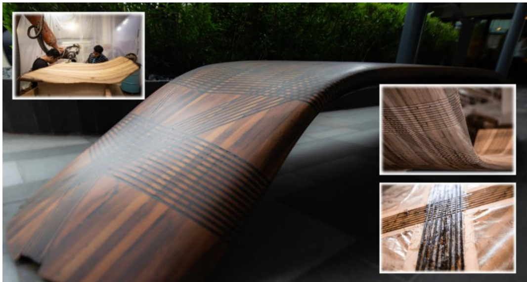
Figure 10. Application of the reinforcement mechanism onto a carbon fiber-reinforced timber bench.
