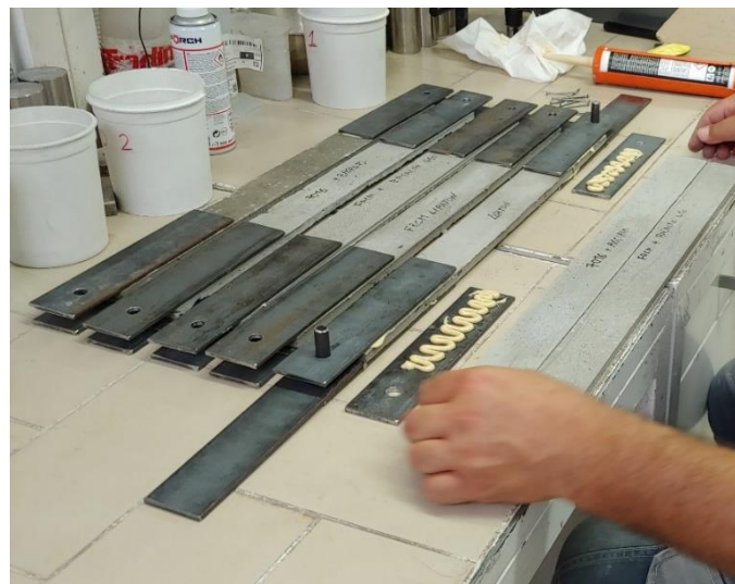
Figure 5. FRCM coupons at the hardened state with steel tabs bonded with epoxy adhesive.
