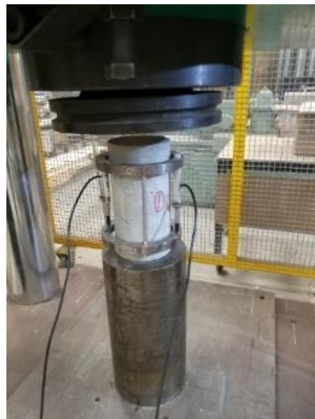
Figure 8. Test device for measuring the compressive stress–strain curve of control mortar.
