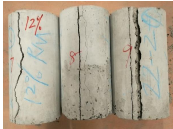
Figure 19. Failure modes of CRM12 specimens.
