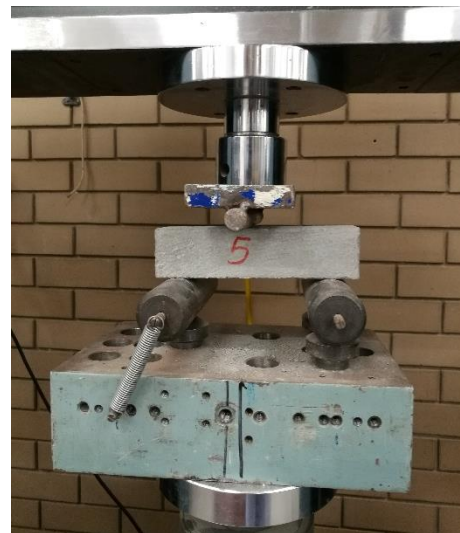
Figure 3. Three-point flexural test setup.
