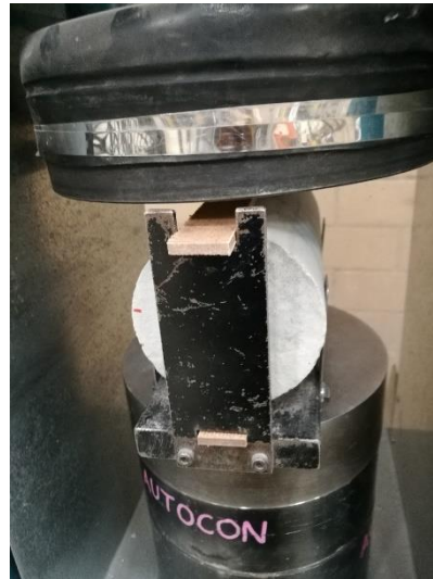
Figure 2. Indirect tensile test setup.
