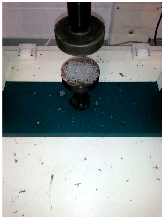
Figure 13. The image shows crushed debris from the FCC lattice around machine jigs after compression.
