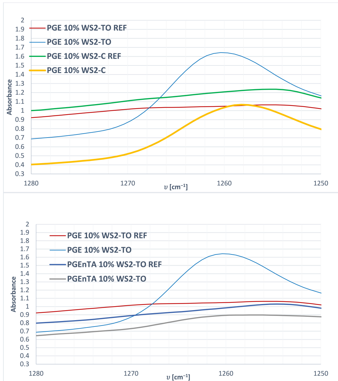
Figure 9. Expanded IR spectrum near the 1260\text{ cm}^{-1} peak for 10 wt.% of WS 2 -TO and WS 2 -C in PGE ( top ) and for 10 wt.% of WS 2 -TO in PGE and PGE n TA. ( bottom ). REF refers to uncured resins.
