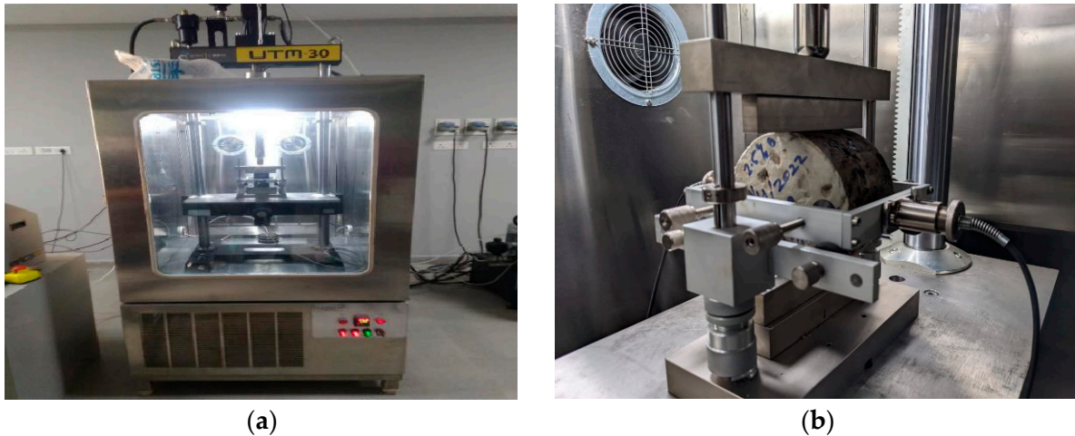
Figure 4. (a) Servo hydraulic cyclic test equipment; (b) cyclic indirect tensile test arrangement.
