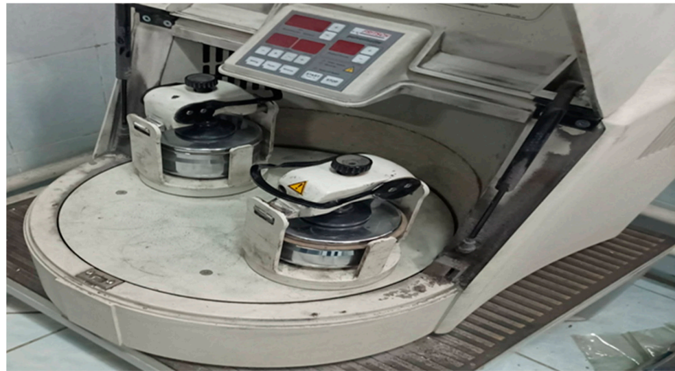
Figure 1. Planetary ball mill (Retsch PM 200F).
