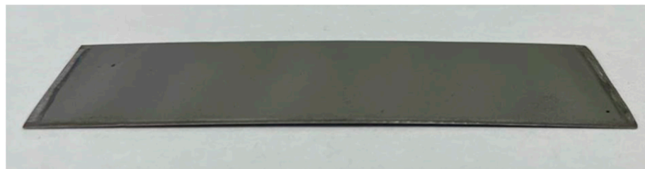
Figure 15. Almen strip with a composite coating produced by spraying the \text{Cu}_3\text{C}_2 powder at k = 1.1 .
