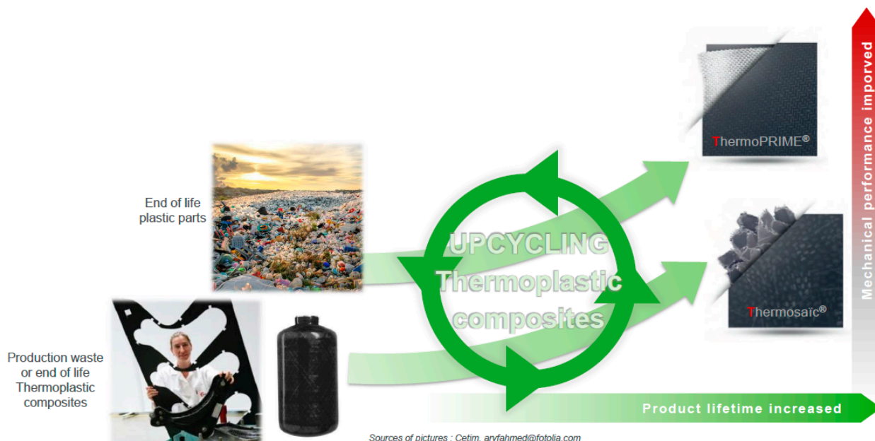
Figure 15. ThermoSaic® Technology to recycle end-of-life tanks [75].
