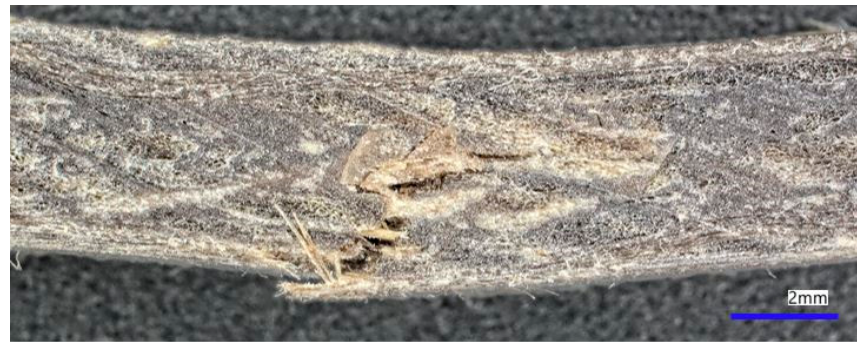
Figure 15. Fracture pattern of a test sample in a three-point bending test.
