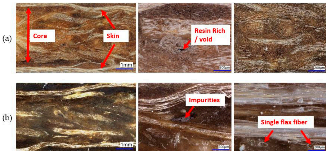
Figure 11. Microscopic images of (a) a sandwich composite panel made using R4 and (b) a sandwich panel made using R10.
