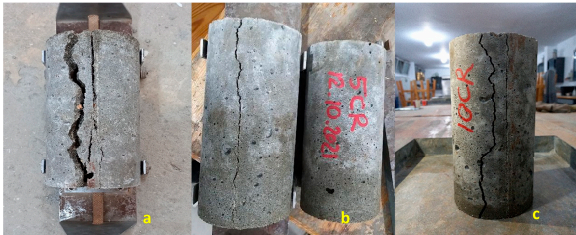
Figure 12. Failure modes of splitting tensile strength for different mixes: (a) control mix, (b) 5CR mix, and (c) 10CR mix.
