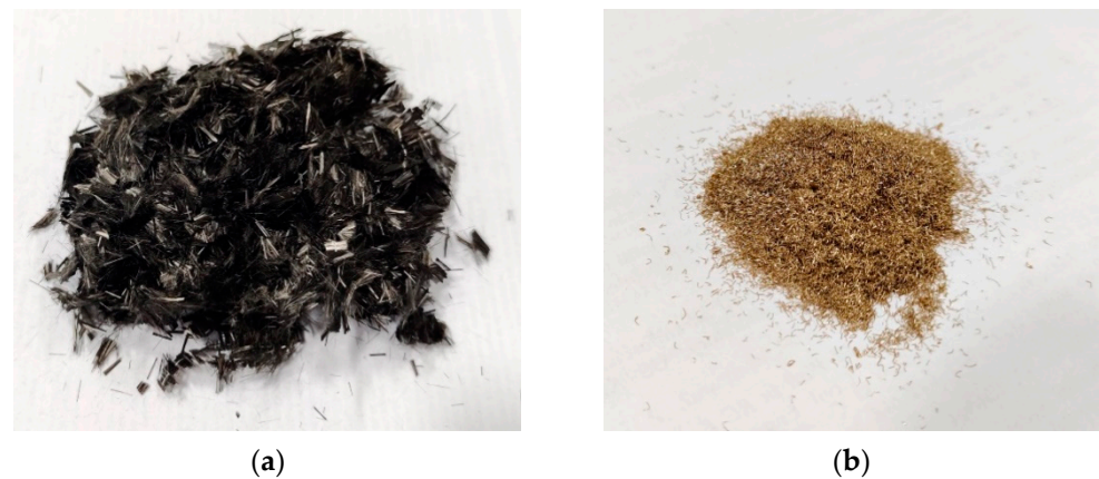
Figure 1. The pictorial representation of brass and carbon fibres. (a) Carbon fibre. (b) Brass fibre.
