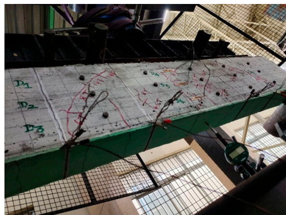
Figure 4. Four-probe method with wire winding on smart mortar.
