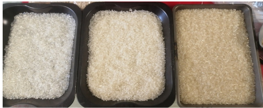
Figure 3. Granulated virgin PLA after recycling process; (Left–Right) 1 recycling, 3 recycling and 6 recycling steps.
