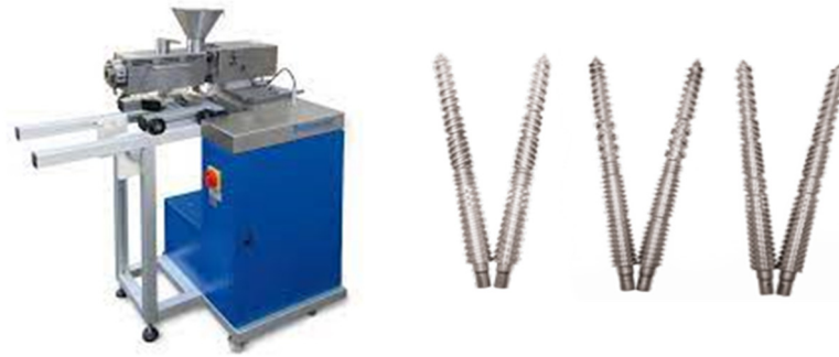
Figure 1. (Left) Brabender conical twin screw extruder and (Right) Co-rotating conical screws.
