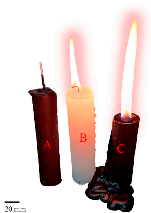
Figure 6. Photo of candles which were made from paraffin/rGO composite (black candle A), paraffin (white burning candle B) and composite (black burning candle C). All candles initially had the same dimensions (diameter 27.6 mm, height 118.8 mm). During the burning time (10 min), the height of the white candle decreased by 9.7 mm, and that of the black candle by 38.4 mm.
