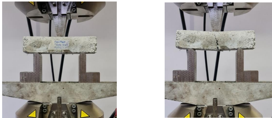
Figure 5. Flexural strength test of mask fiber mortar beam.
