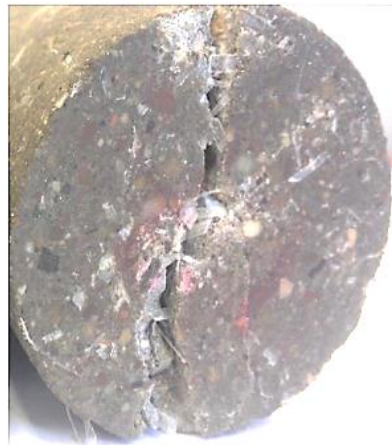
Figure 4. Failure of mask fiber mortar at split tensile test.
