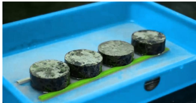
Figure 7. Sorptivity test on mortar.
