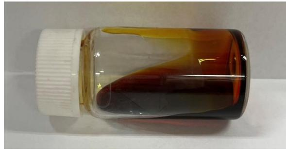
**Figure 7.** Obtained viscous gel electrolyte.
