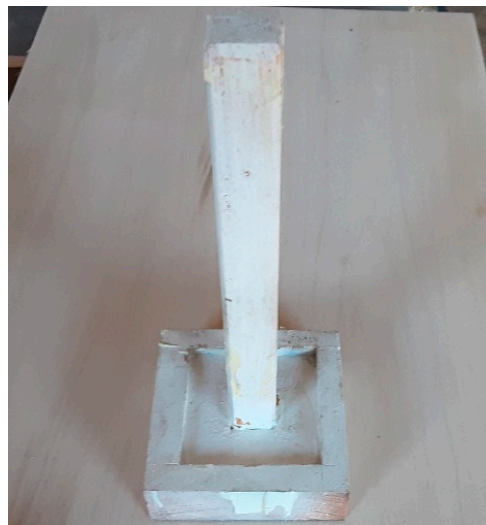
Figure 2. The base of the mold, which features a square dowel to allow for supporting the PVC inner-core during fabrication.
