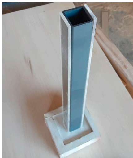
Figure 3. The glass and inner core have been installed onto the base.
