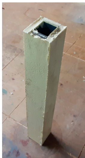
Figure 5. A column after casting showing the hollow core. Note the additional polyurethane resin left at the top of the column, which is present on both ends.
