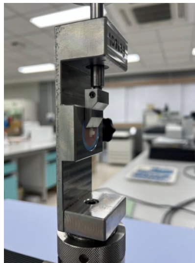
Figure 2. The knife-edge SBS test.
