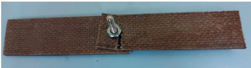
Figure 6. Fractured lap joint 4MHJC specimen.
