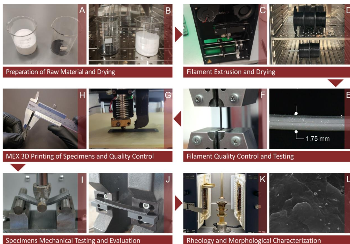
Figure S1. The experimental procedure's workflow: (A) raw materials; (B) drying process; (C) filament extrusion; (D) filament drying; (E) filament quality control; (F) filament mechanical testing; (G) samples 3D printing; (H) samples inspection; (I) samples mechanical testing (three-point-bending); (J) samples mechanical testing (impact test); (K) rheology testing; (L) morphological analysis with SEM.
