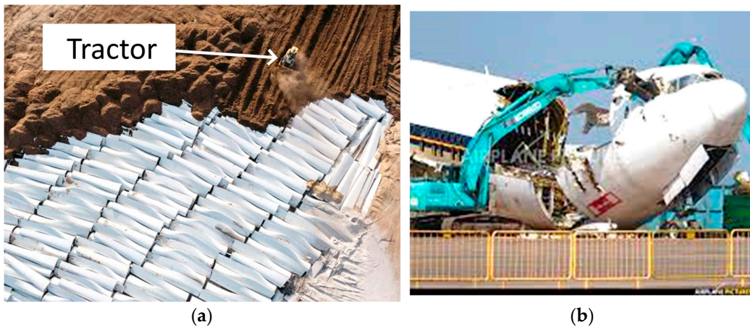
Figure 2. (a) Decommissioned wind turbine blades awaiting landfilling. Note the tractor at top right for scale. Adapted from [14], used with author’s permission. (b) Scrapping of a Boeing 777 airliner during the Covid pandemic. Picture from [15], used with author’s permission.
