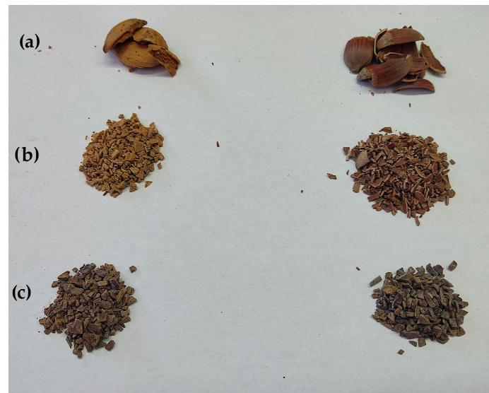
Figure 1. Waste almond and hazelnut nutshells: (a) as received waste nutshells, (b) ground waste nutshells, or (c) nutshells treated with milk of lime for 2.5 h at 80 °C.
