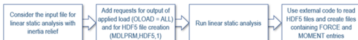
Figure 9. Flowchart for calculation of loads equivalent to inertia relief loads.
