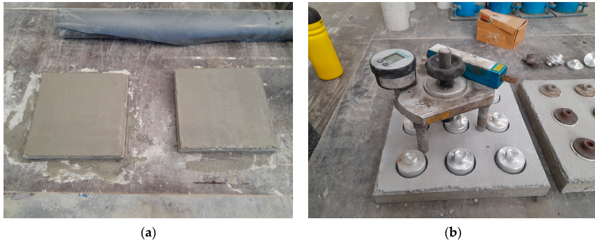
Figure 2. Tested samples: (a) protective modified mortar applied; (b) test samples during the pull-off tests.
