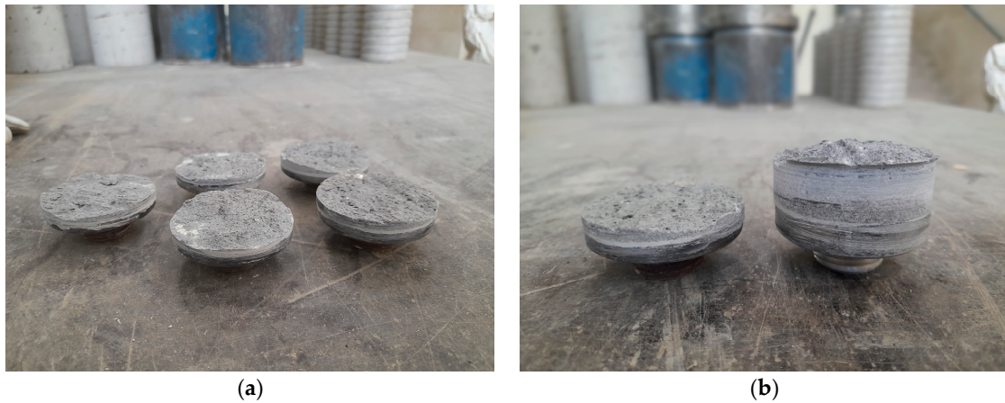
Figure 7. Rupture of samples after pull-off tests: (a) in mortar; (b) in mortar and concrete.
