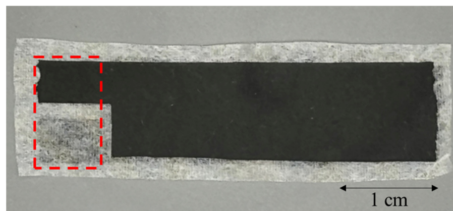
Figure 6. Constructed paper actuator. The dotted box indicates the area where the wooden clip for the voltage input clips in. For ease of viewing the structure, the actuator in this figure does not contain ionic liquid.
