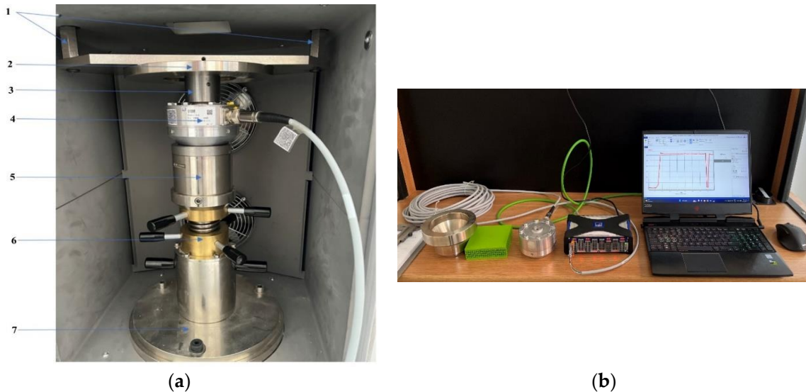
Figure 8. Measurement setup of the force pressing the sandwich panel: (a) load fixture and (b) measuring system of the force.
