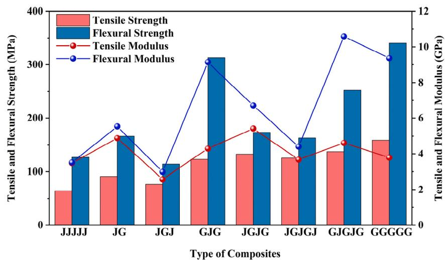
Figure 5. Tensile strength, flexural strength and modulus of E-glass fiber (G) and jute fiber (J) composite laminates.
