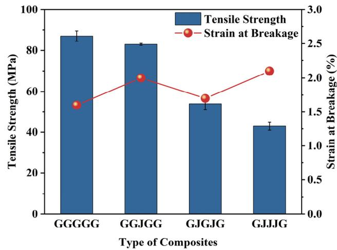
Figure 4. Tensile strength and fracture strain of E-glass fiber (G) and jute fiber (J) hybrid composite laminates.
