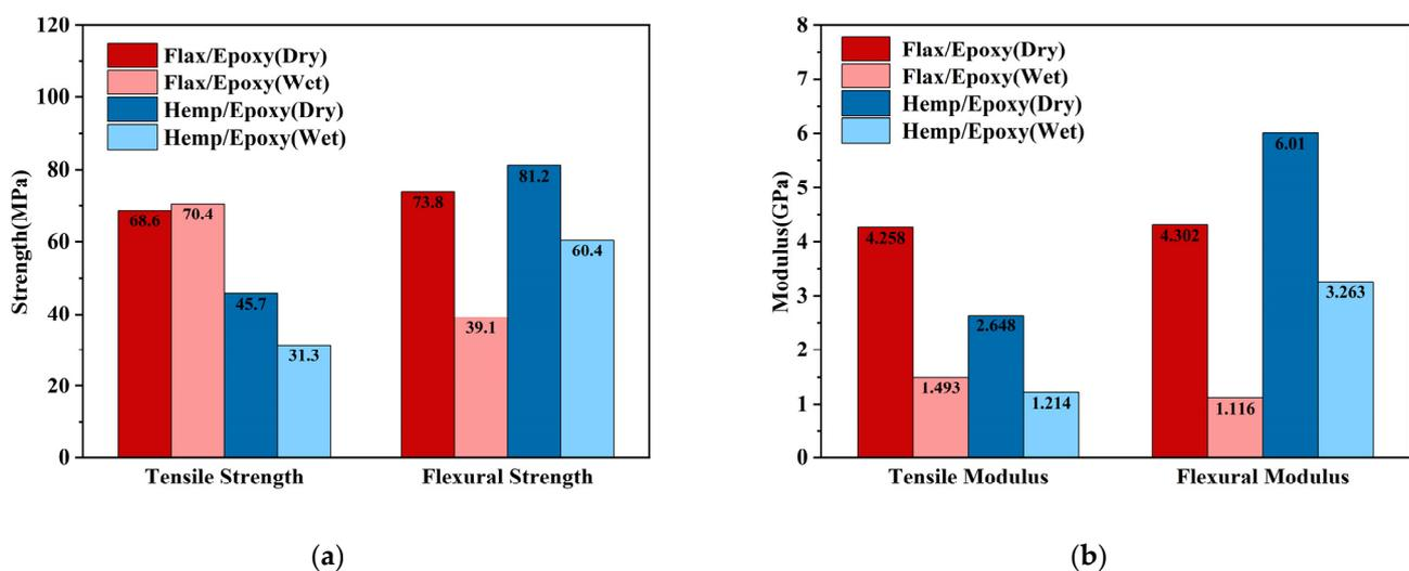
**Figure 8.** Mechanical properties of Flax/Epoxy and Hemp/Epoxy: (a) Strength changes under wet and dry conditions; (b) Modulus changes under wet and dry conditions.
