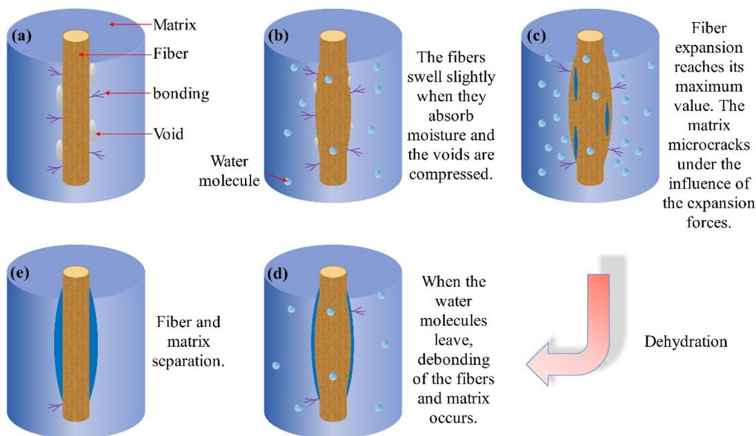
**Figure 7.** The influence of water in the interface between fiber and matrix: (a) Initial state before water absorption; (b) Moisture absorption process; (c) Saturation state; (d) Drying process; (e) Dry state after moisture absorption.
