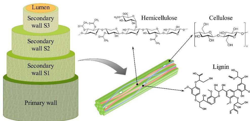
Figure 3. Structural composition of the cellulose fiber.
