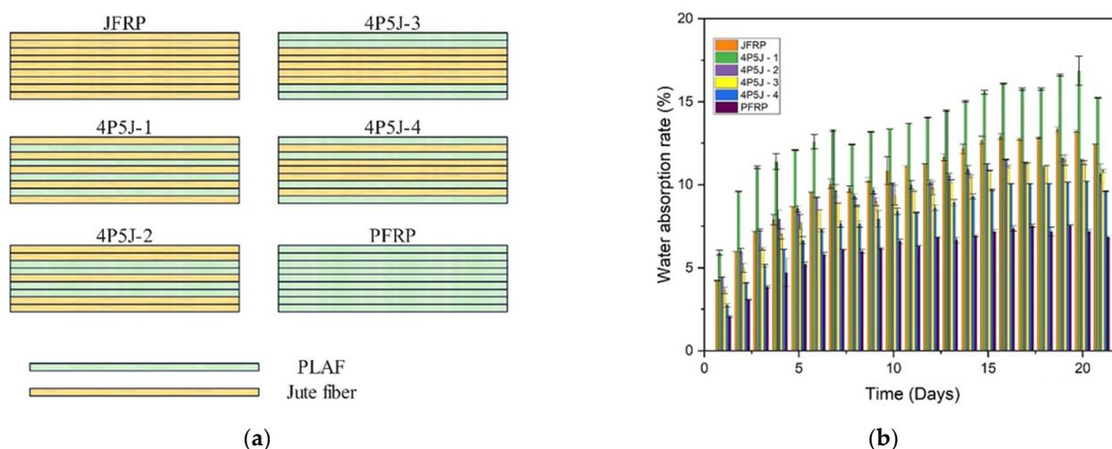
**Figure 6.** Hybrid natural fiber-reinforced composites uptake water test: (a) Stacking sequence and nomenclature of biocomposite laminate; (b) Moisture absorption rate after immersion in water at indoor temperature (Reproduced with permission from [73], Elsevier, 2023).
