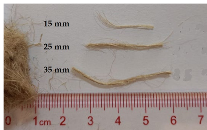
Figure 4. Used lengths of fibers in preparation of geopolymer concrete specimens.
