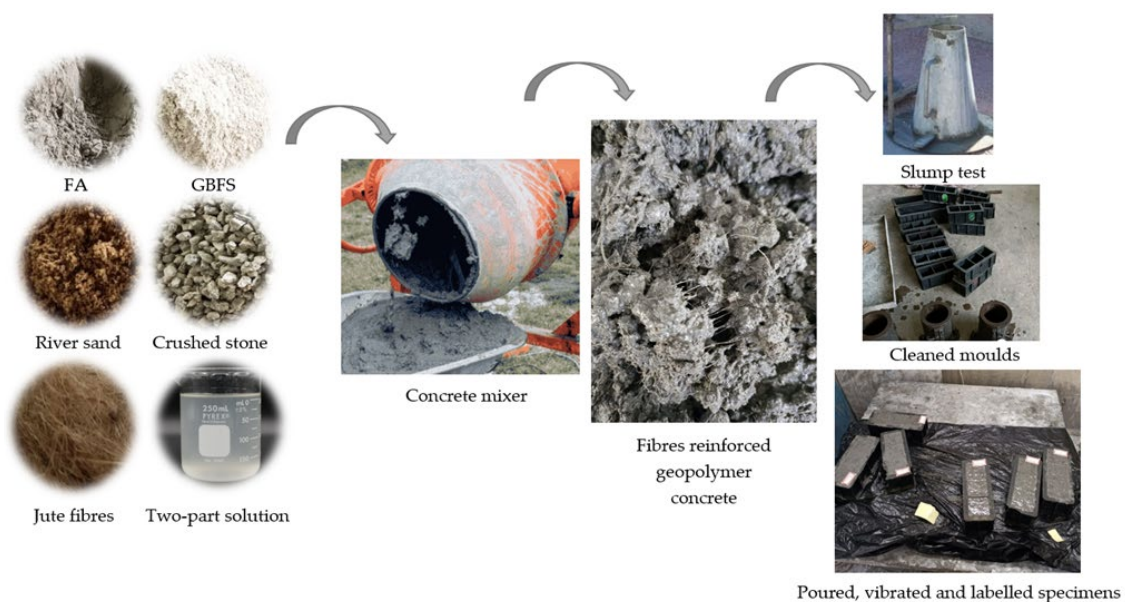
Figure 6. Jute fiber-reinforced geopolymer concrete specimens' preparation.
