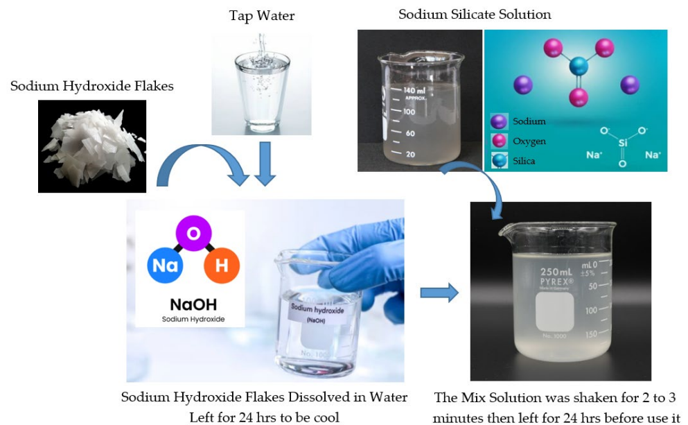
Figure 2. Protocols of alkali activator solutions preparation (two parts).
