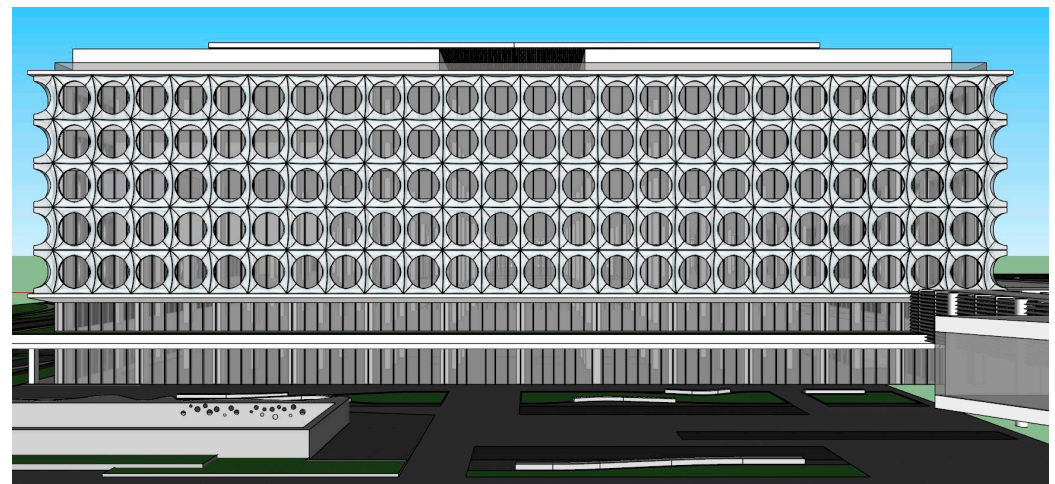
Figure 2. Building surrounded by periodic GPL/ETFE composite tensile membrane units.
