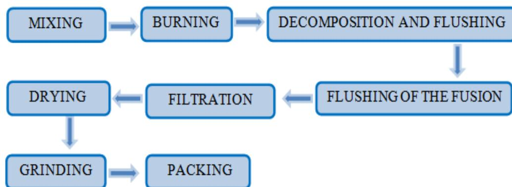
**Figure 1.** The flow chart diagram of pigment synthesis.
