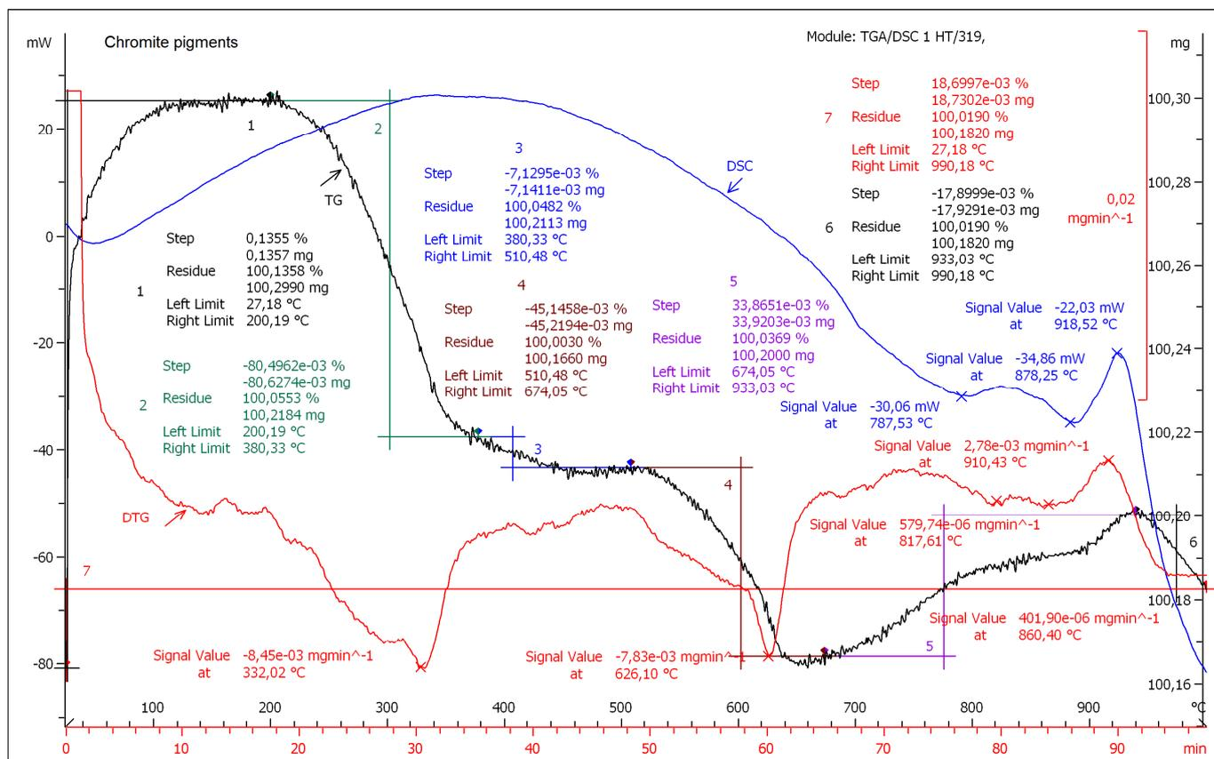
Figure 3. Thermogravimetric analysis of chromite pigments.
