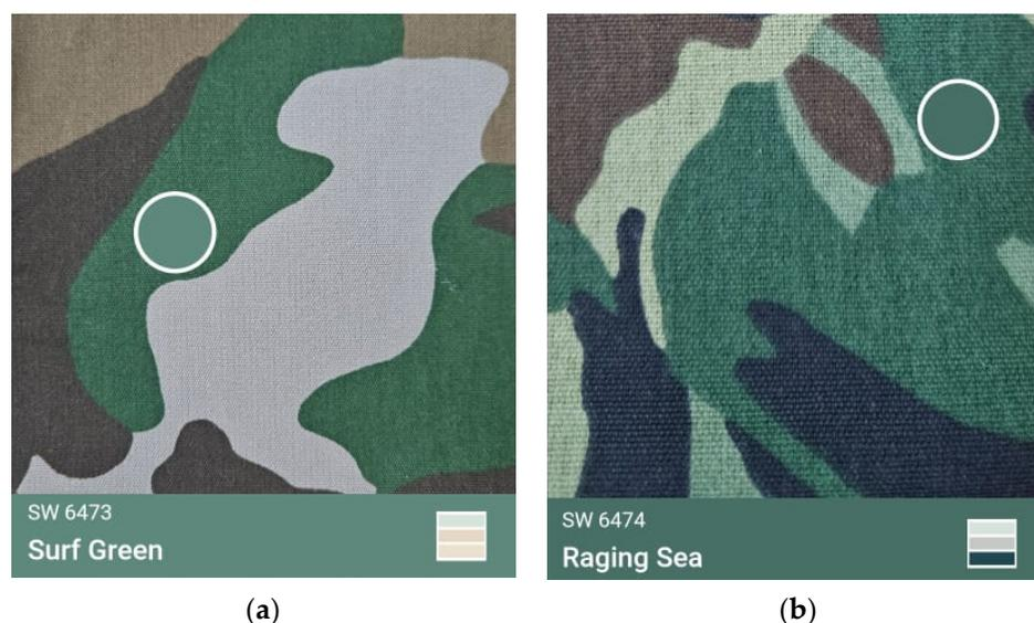
**Figure 6.** Samples of fabrics with applied pigment from technogenic wastes. (a) Cotton fabric Alatau article 1001. (b) Composite fabric Arlan article 6005.
