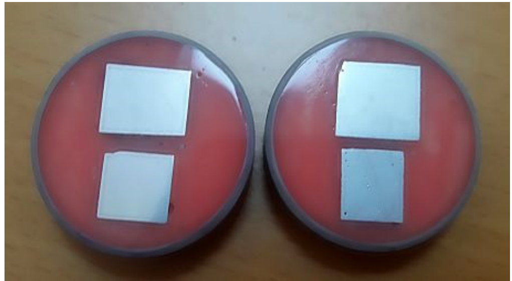
Figure 3. Specimen set in wax molds for microstructural examination.
