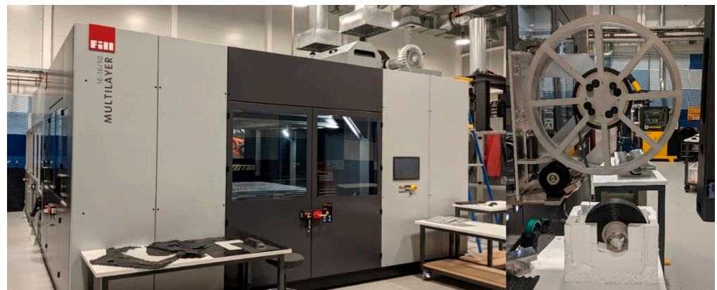
Figure 1. Reference photo of the Fill Multilayer during tape-laying operations and CFRP winding from a roll to a cassette.
