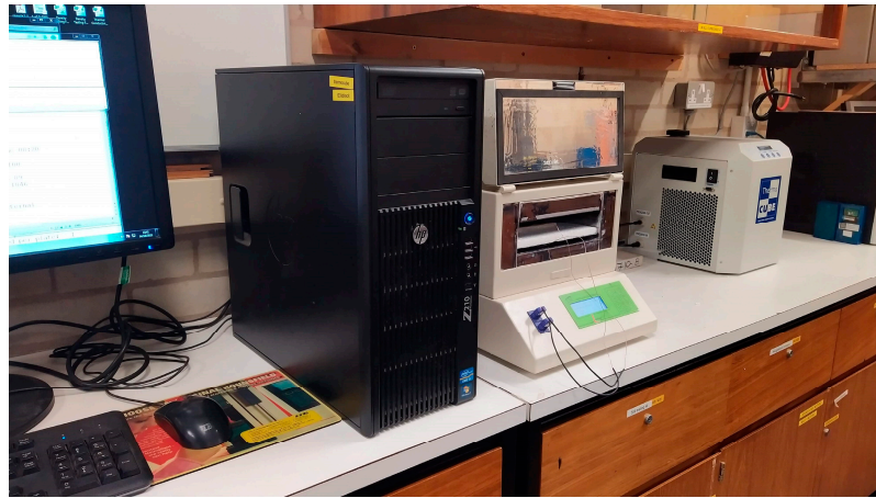
Figure 2. FOX200 apparatus by LaserComp for thermal conductivity testing.
