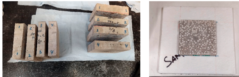
Figure 3. Sample preparation for thermal conductivity testing.
