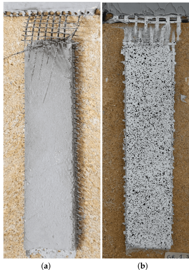
Figure 11. Failure of textile (E1): (a) specimen BC_DSB_1; (b) specimen GC_DSB_2.
