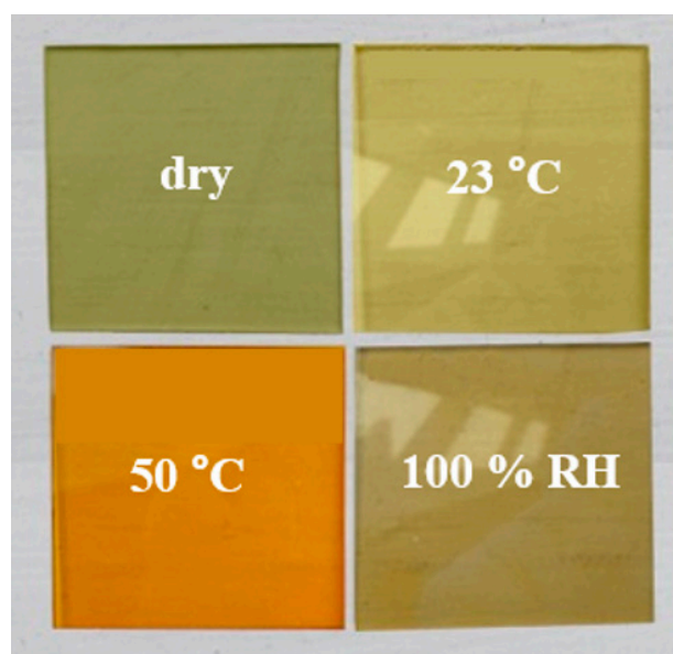
Figure 2. DION 1260 SM60 polymer colour changes under different ageing conditions.
